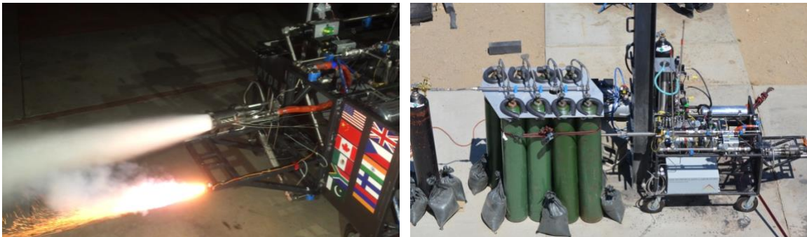
Figure 12. Preparation for Jessie inaugural static fire. a) Hydra timing test b) Test stand setup
