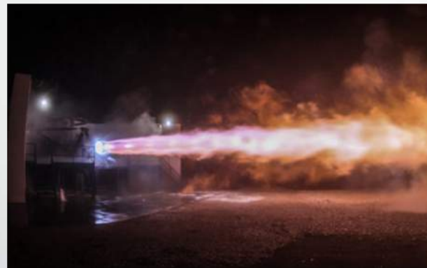
SpaceX Raptor Engine Liquid Methane / LOX ISP vac = 360 sec Exhaust Color: "Purplish"
