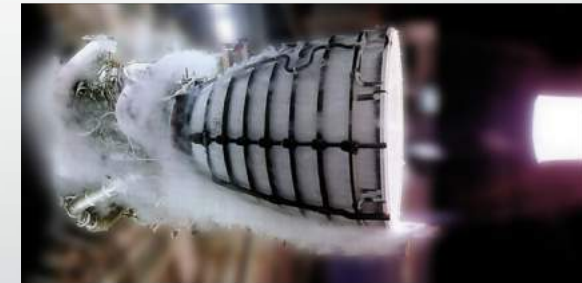
Space Shuttle Main Engine Liquid Hydrogen / LOX ISP vac = 450 sec Exhaust Color: "Clear"
