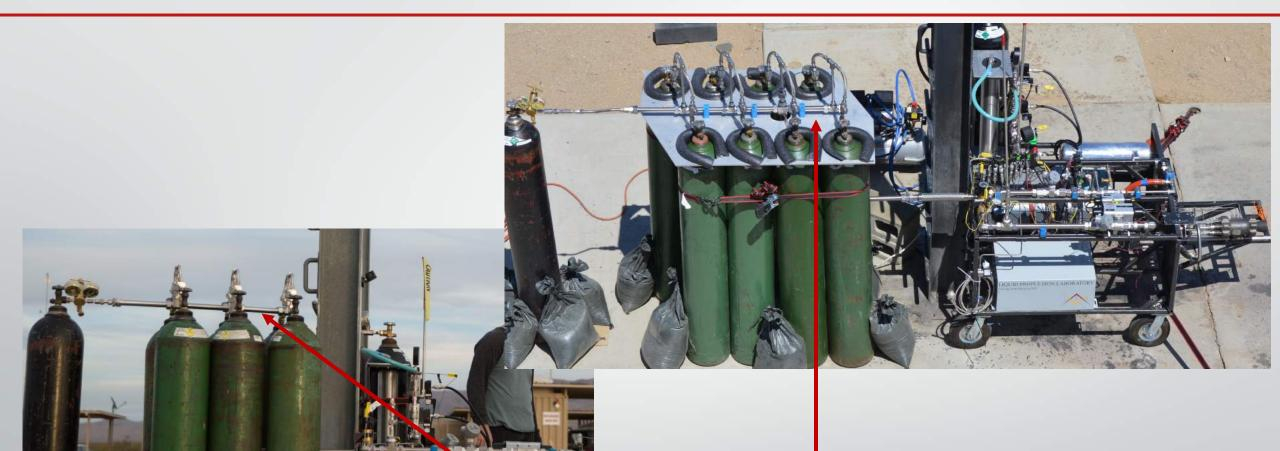
New oxygen manifold to ease assembly & increase oxygen cylinder capacity from 6 to 8
