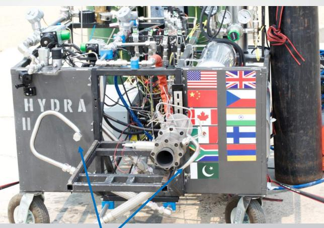
Propellant feed lines modified for dual engine firing capability
