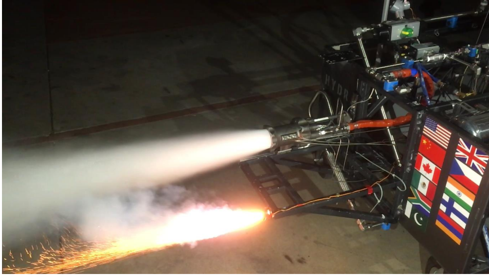
Fig. 17 Image of slow motion video showing the timing test conducted for the Jessie engine.
