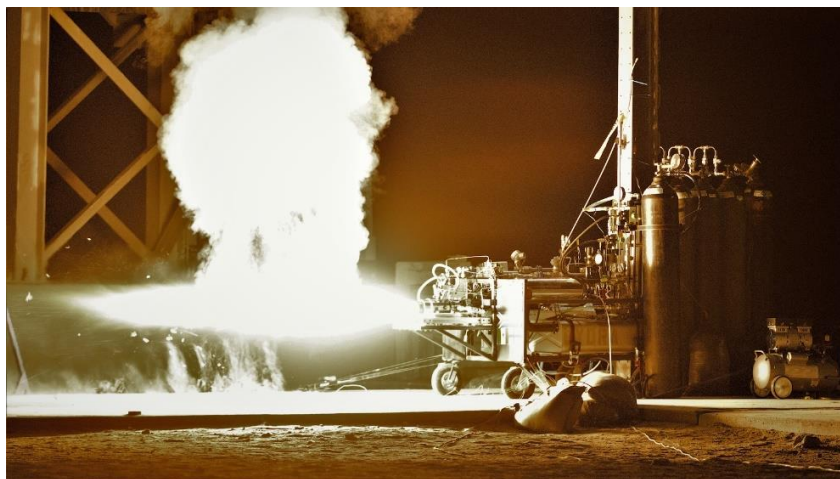
Fig. 19 Blue Steel 2.0 Engine (Kerosene and GOX, 500 lbf thrust, 6 second duration).
